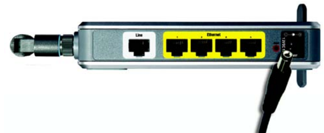
Figure 4-3: Connect the Power
